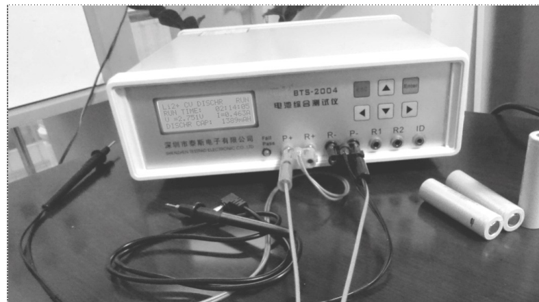
Fig.2. Measuring apparatus: battery tester - charger/discharger BTS-2004
